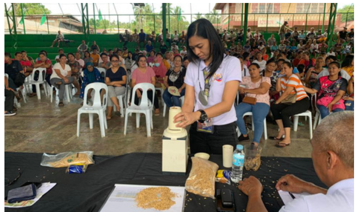
BSQAO Arajo demonstrates the process on drawing out the palay's moisture content using the moisture meter
